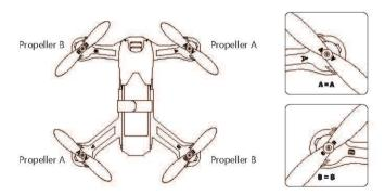
Installation: Before installing propellers for the first time, please check that each Propeller A is matched with motor A and each Propeller B is matched with motor B. Align the "I" with the flat side of the "D" shaped motor shaft. Then use the provided screws and screwdriver to secure each propeller. Propeller A's are paired with black propeller screws and are tightened counterclockwise. Propeller B's are paired with silver propeller screws and are tightened clockwise. (as shown below)
