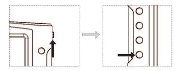
3. Connect the drone to its battery. While all units are in either binding or pairing modes, please do not touch, press or move any of the transmitter joysticks, buttons or keys. Doing so will cause the aircraft to drift or perform unstably during flight. After binding is successful, the transmitter's binding status LED will be a solid blue.
