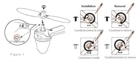
Note: Mind the differing colors of the A and B propeller screws!
